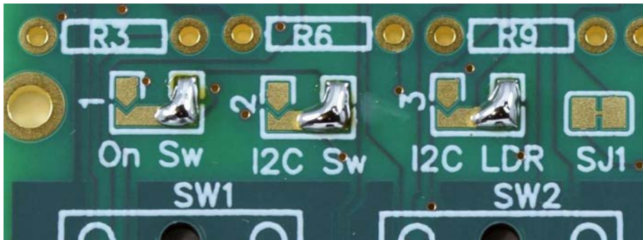
Fig. 7. Three solder bridges must be made.
