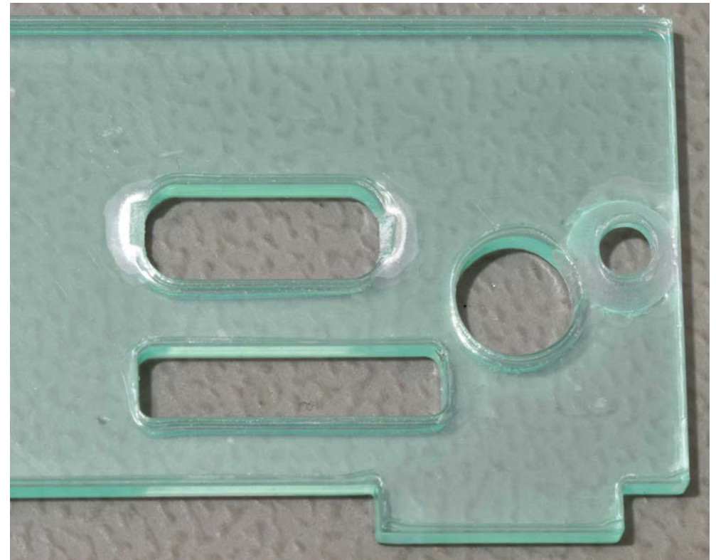
Fig. 19. Some filing out of the USB-C-socket mounting hole.
