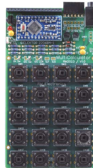
Fig. 12. 20 switches for testing.
