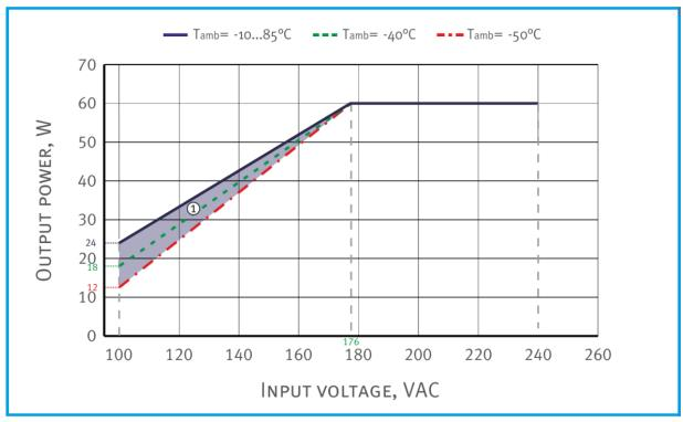
1 - For ambient temperature -50°C...-10°C in gray areas of diagrams some specification parameters may not be met.
