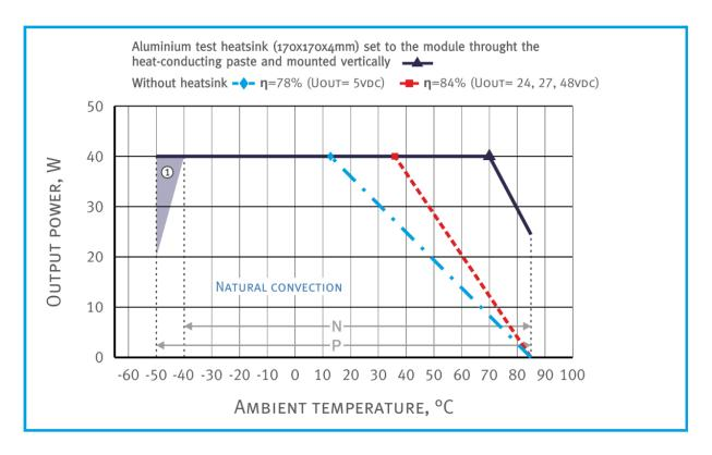
Dropping parts of the dashed and dash-dotted curves are in accordance with the **maximum temperature of the case** (for modules with index <N>, <P> equal to +85 °C). Output power must not exceed the values which are limited by corresponding curve for a given ambient temperature.
