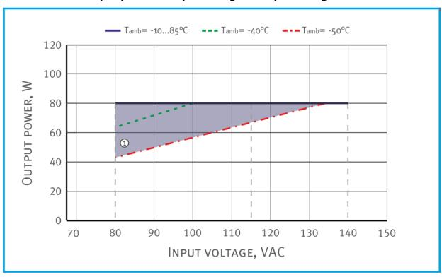
① - For ambient temperature -50°C...-10°C in gray areas of diagrams some specification parameters may not be met.
